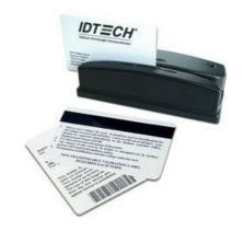
The rugged Omnireader swipe reader reads barcodes and/or magnetic stripes. With its metal base and durable plastic case, it can be used even in rough environments.
